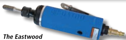
The Eastwood straight die grinder is outfitted with a Harbor Freight 1/4-inch brass air hose connector while a 3-inch Eastwood Carbide burr is ready for use.
